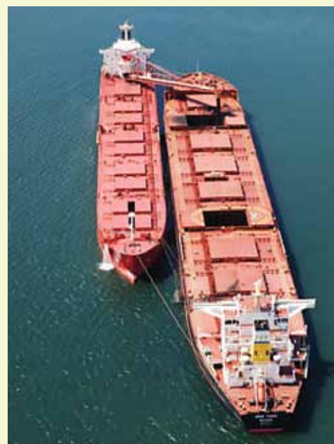
CSLI Pool vessel Bernhard Oldendorff tops off the Capesize New York in the Strait of Canso, Nova Scotia.
